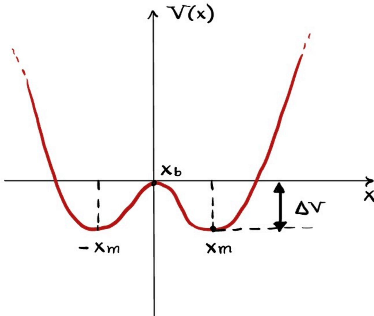
$$m \frac{d^2 x}{dt^2} = -m \gamma \frac{dx}{dt} - \frac{dV(x)}{dt} + \underbrace{m A_0 \cos(\Omega t)}_{\text{forzante}} + \underbrace{B \xi(t)}_{\text{fluttuazioni stocastiche}}$$
