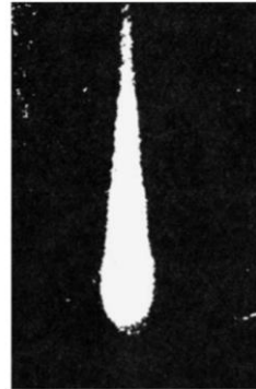
Drop-like shape of an avalanche Left: cloud chamber picture Right: schematic view
