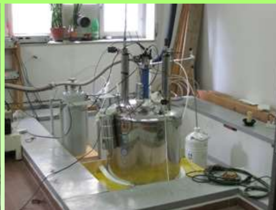
9 Tesla magnet for broad-band NMR
