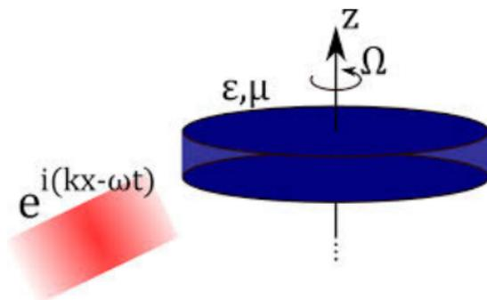
$$F^{\mu\nu} = \begin{bmatrix} 0 & 0 & 0 & E_z \\ 0 & 0 & 0 & -B_\phi \\ 0 & 0 & 0 & \frac{B_r}{r} \\ -E_z & B_\phi & -\frac{B_r}{r} & 0 \end{bmatrix} \implies \begin{cases} \mathcal{B}_\phi = -\frac{i}{\omega} \frac{d\mathcal{E}_z}{dr} \\ \mathcal{E}_z = \frac{\Gamma}{\omega} (\omega - l\Omega) f(r) \\ \mathcal{B}_r = \frac{\Gamma}{\omega r^2} (l - \omega\Omega r^2) f(r) \end{cases}$$
